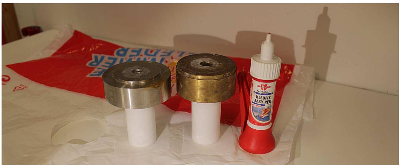
Figure 3. Gluing 150 $\mu$  plankton mesh (nylon) to the bottom of the incubator unit using superglue (cyanoacrylate).
